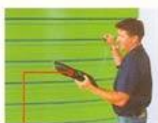
Ultra-sounding of tanks for additional quality control
